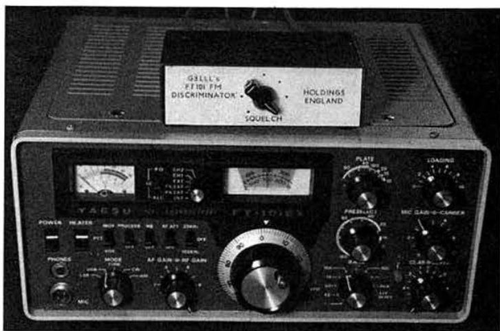
The fm discriminator mounted on top of an FT101
